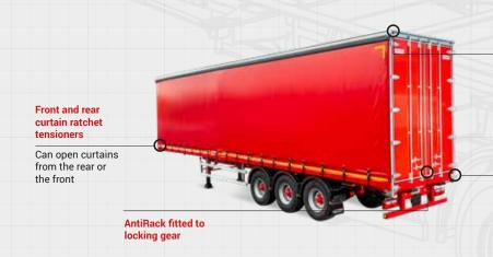
Galvanised rear door pillars and 34mm diameter locking gear
